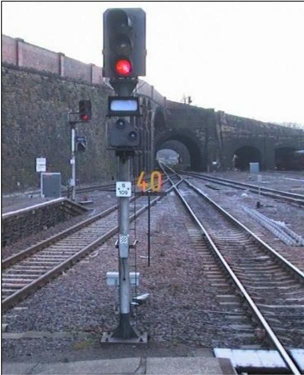
UK standard 3-Aspect Signal at Sheffield (Midland). Below the red aspect is a sign which, if the signal is showing a proceed indication, illuminates "RA" (Right Away) to tell the driver station duties are complete and he can start the train. Below this is a shunt signal, which carries no red light in this case as the red is already available on the main signal. The signal carried a white identification plate and, nearer the ground, a signal post telephone. Photo: Author.
