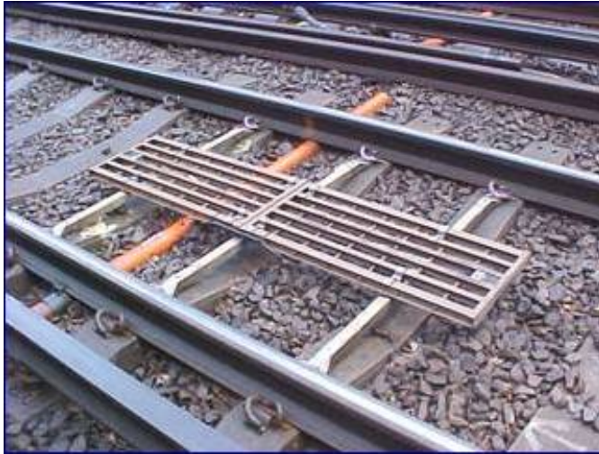
Figure 9: A pair of TPWS loops fixed to the track close to a signal. The two loops act as a tripping activator if a train attempts to run past a signal showing a stop aspect. Most main line signals in the UK are fitted with this system. There will also be two further loops on the approach to the signal set to match the required train approach speed. Photo: Author's Collection.
